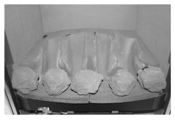
d) Select four of the large coals and arrange behind the front row of coals, ensuring that flame paths as indicated below are not interupted, place one of the small coals at each end of the second row. (See fig. 6 below)
